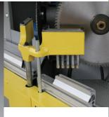
Self-Adjustable Vertical Pneumatic Clamping System
